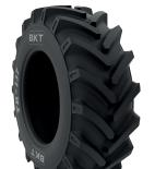
TR 137 is BKT's most suitable tire for all harvesting operations. It ensures excellent traction in the fields even with high loads. The tire is available in different versions: the "aramid-belted" version provides better puncture resistance and protection against all typical damages of this application; the "HD" version provides extraordinary cut and chip resistance, and an extended tire life-cycle.
