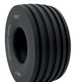
RIB 775 is a low-section cross-ply tire for transport and soil tillage applications with trailers and implement machinery. It offers great load capacity and a long tire life-cycle.
