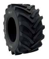
MULTIMAX MP 515 is an agro-industrial radial tire designed for universal vehicles and fertilizer trucks. It is suitable for municipality and transport applications. The tire shows a unique tread design providing superior riding comfort on the road as well as excellent self-cleaning properties and great traction. The strong steel-belted nylon casing and the reinforced shoulder ensure extraordinary durability. MULTIMAX MP 515 is the perfect tire also at high speeds (90km/h).
