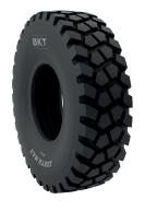
EARTHMAX SR 33 is a radial tire for multipurpose trucks. Its multi-block tread pattern has been specially designed to guarantee extraordinary traction on soft, sandy, or muddy surfaces. EARTHMAX SR 33 provides outstanding stability in addition to best self-cleaning properties. The strong All Steel casing features excellent durability and resistance to snag and punctures.
